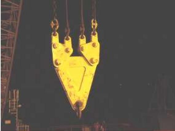
In a 4-rope crane, the winches are automatically locked together so that the holding and closing lines work together without operator input.
