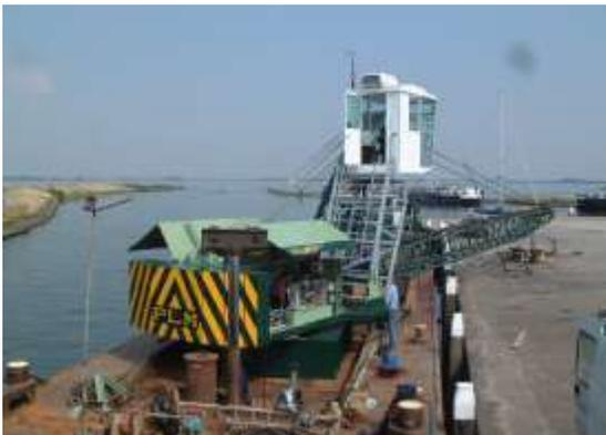
The side panels of the crane are raised hydraulically and cover the mechanic to protect from the elements. Lights are provided inside the covers. PLM Cranes are designed for ease of maintenance. PLM offers a diagnostic package with the electronic control option that allows the mechanic to connect a pc or dial up from remote location to diagnose the crane. PLM is able to diagnose your crane remotely from the factory.
