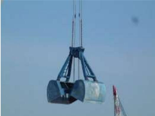
The clam is stable and does not require a tagline. This is important for unloading ships where the tagline rubs on hatch coamings and in dredging operations where the clam extends well below the base of the crane. In standard configuration, a 4-rope crane can dig as much as 100ft below the base of the crane. The boom hoist is designed to take the rope on one layer of the drum and is designed for continuous high speed booming needed in clamshell work and breakbulk.
