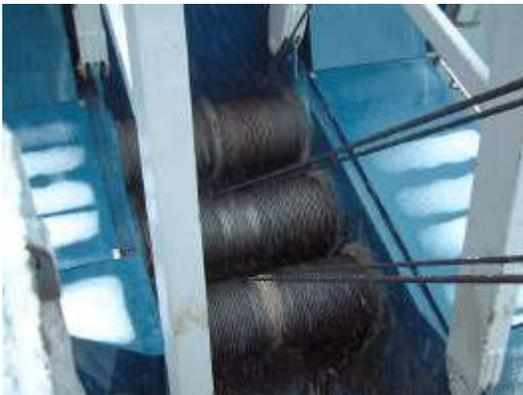
The photograph above illustrates the concept. Note two ropes coming from each drum, one from the right which is a right lay rope and one from the left which is a left lay rope. The ropes go straight up the boom over very large diameter sheaves down to the clam.
